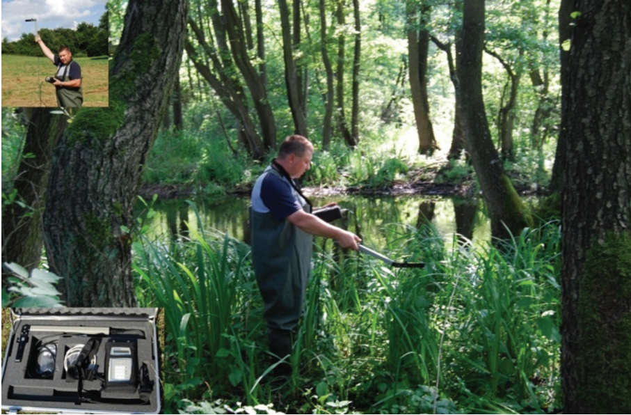
Ryc. 8. Pomiar indeksu LAI Fig. 8. Measuring of the index LAI
